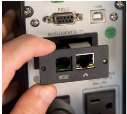
3. Plug the network cable to the Ethernet port.
