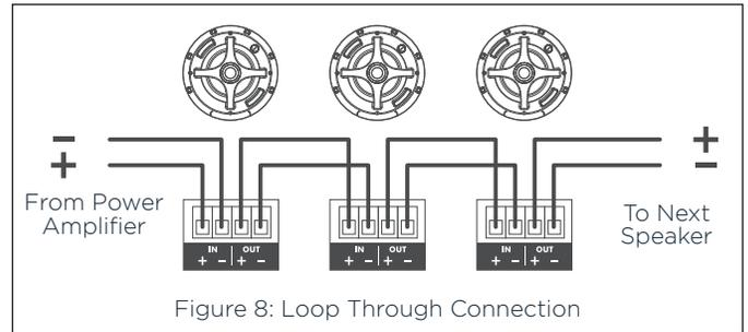
Figure 8: Loop Through Connection
