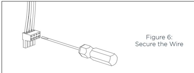
Figure 6: Secure the Wire
