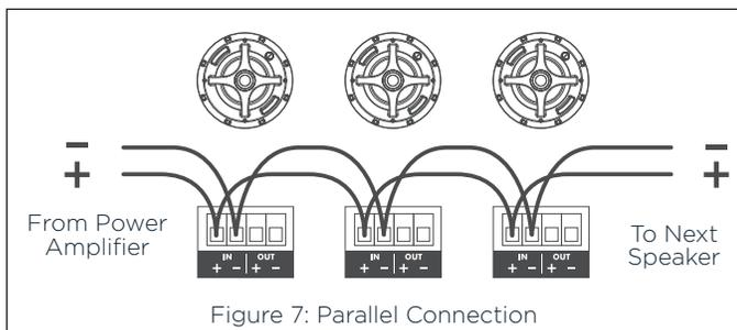
Figure 7: Parallel Connection
