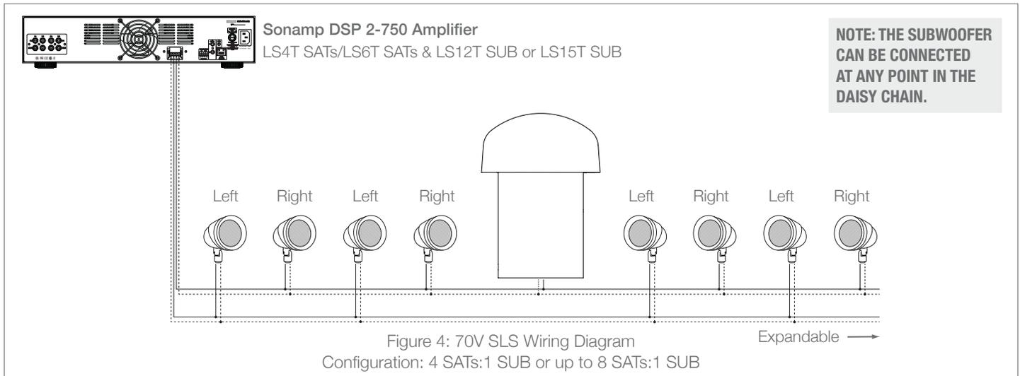
Figure 4: 70V SLS Wiring Diagram
