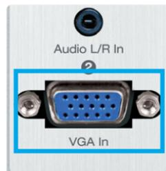
› **Analog Audio Input:** Using a 3.5mm stereo cable, connect your audio source to be associated with the VGA video input.
