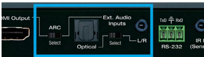
› **ARC Select and External Audio Input Select Switches:** Choose which audio to return from the Rx to the Presentation Switch:
