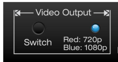
There is a black pushbutton to toggle between the two output resolutions. The LED next to the pushbutton will change color to indicate the selected resolution.
