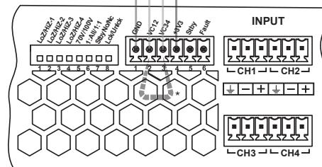
\*Short the two VC inputs to control all channels
